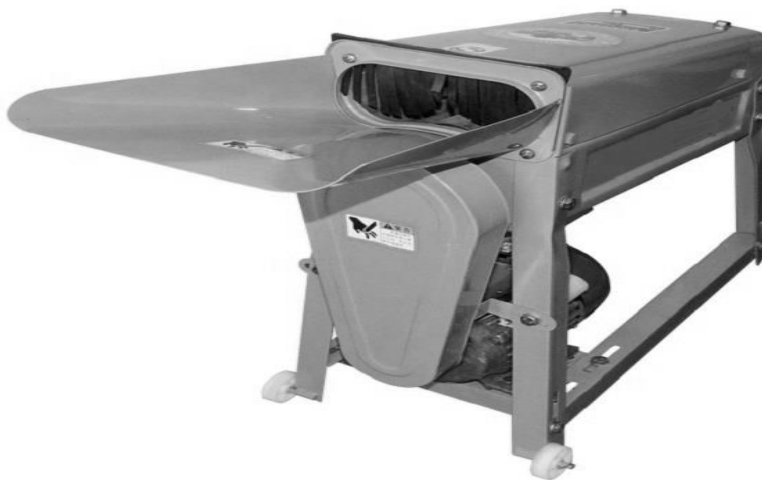
Figure 1 Machine (type 5TY-31-86) used for sheller maize
